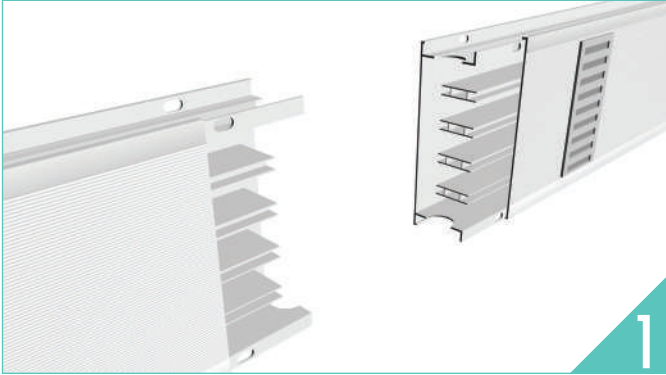
1) Ek eleman yan plastiklerini monte ediniz. 1) Assemble side covers of joint points.
